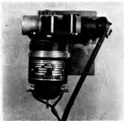
Fig. 5B. Close-up of calibrating unit mounted in front of photocell.
